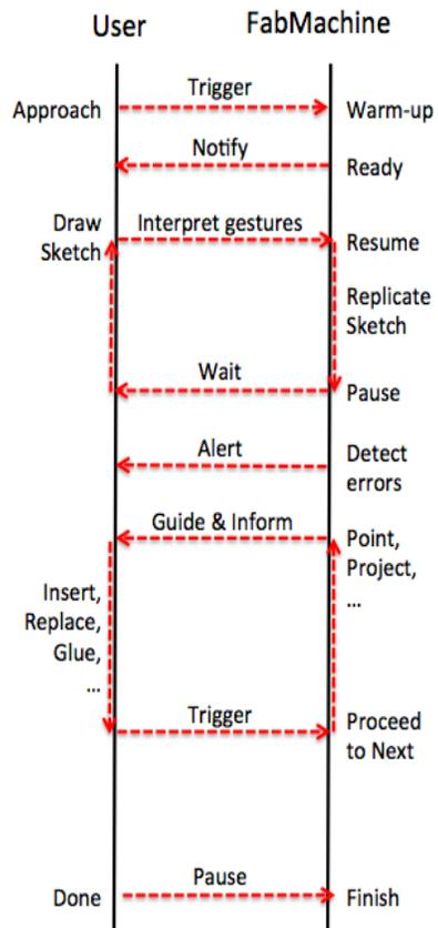
**Figure 5.** A possible exchange of task leadership, where the human has control and leadership at each stage of co-design process. From the preparation of the virtual model to holding the final physical artifact in hand, the user and a fabrication machine collaborate, dealing with problems, materials, and partial representation of outcomes.
