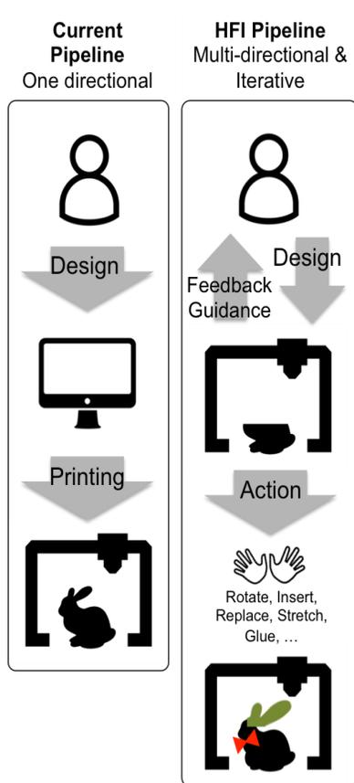
**Figure 4.** A re-imagined of a 3D printing workflow from the vantage of HFM Interaction. This proposed multi-directional process allows the user to modify their design during production, allowing for spontaneous decisions and ideas to be incorporated without needing to begin production from the beginning.
