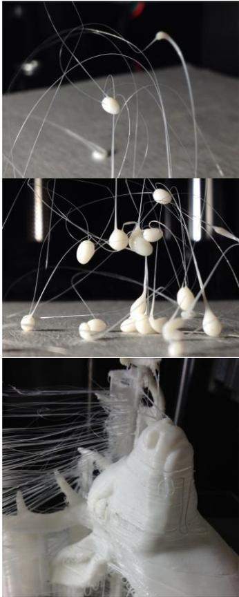
**Figure 2.** Through failed attempts working with his 3D printer, an artist discovered the “beautiful accident” printing technique. Such serendipitous ‘accidents’ could be exploited to inject aesthetics or enhance the textures of computationally fabricated artifacts.
